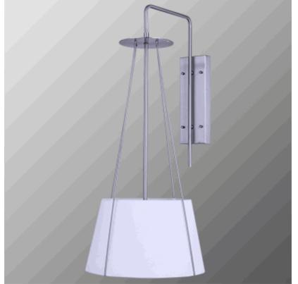
31.75" Brushed Nickel Wall Lamp, one GU24 socket, NO Switch, Direct Wire, with 10.5 x 14 x 8.5 White Linen Hardback Shade with white acrylic bottom diffuser. Recommend 1100 lumen LED bulb with GU24 base.
